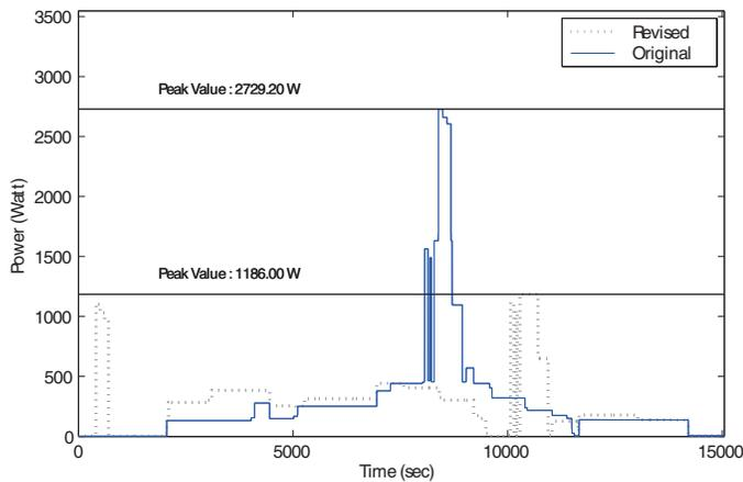
Fig. 14. Comparing power consumption patterns of the two schedules shown in Fig. 13.
