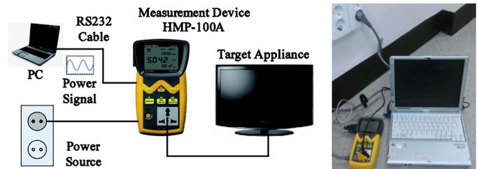
Fig. 11. Measuring power consumption of home appliances using HMP-100A (Adpower Co., Korea) [20], which allows the user to store the measurement data into a computer.
