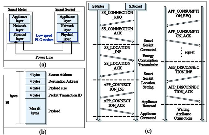
Fig. 9. Details of the communication between Smart Meter and Smart Socket modules. (a) Protocol layers (b) Packet definition (c) Packet exchange diagram
