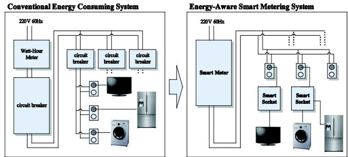
Fig. 5. A conventional system (left) versus a next-generation system with smart metering supported (right).
