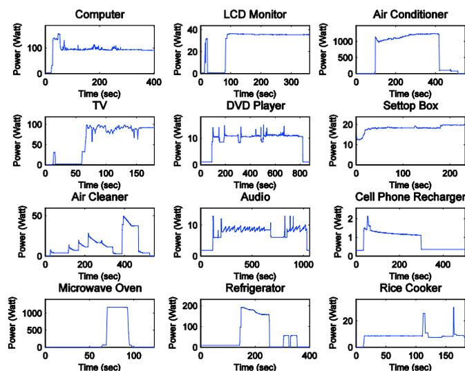
Fig. 1. The power dissipation patterns of typical home appliances.
