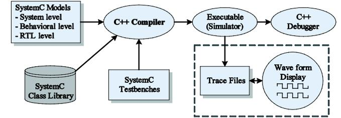
Fig. 7. Simulation flow in SystemC [15].
