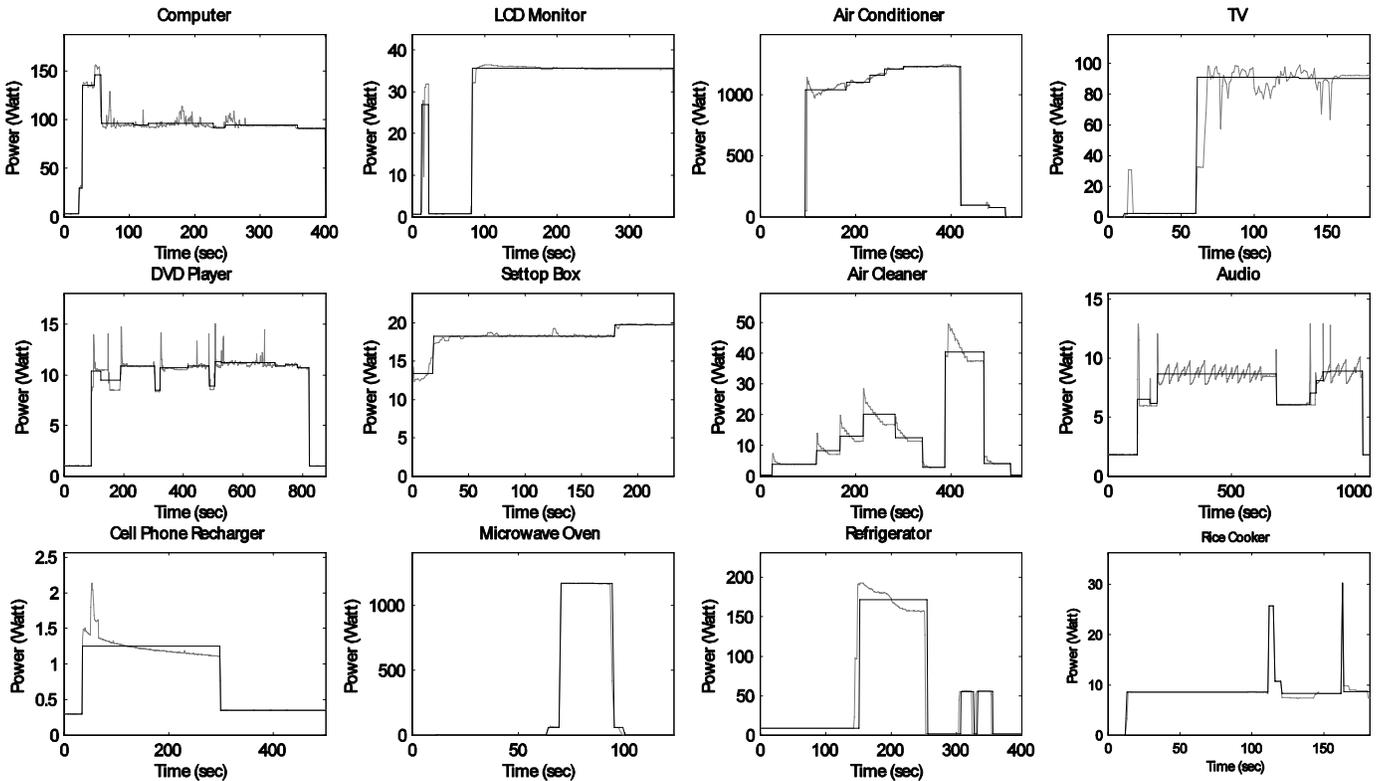
Fig. 12. Comparison of actual (gray) and simulated (black) waveforms for 12 different appliances.
