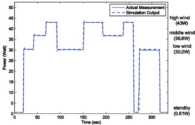
Fig. 8. Four operational modes of an electric fan (model: EFE-434R, Hanil Electric Co., Ltd., Korea) and the corresponding power consumption.
