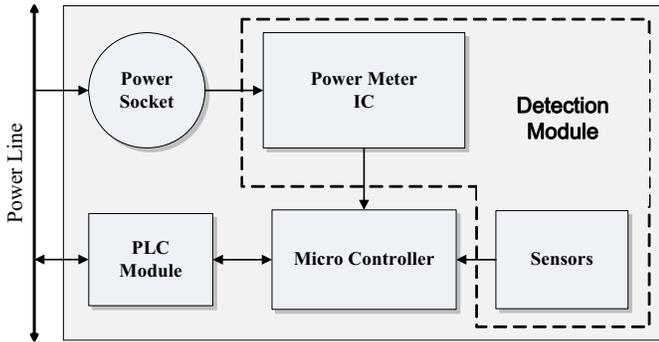
Fig. 4. The block diagram of RMCPS [12].
